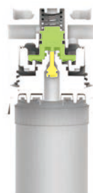
QTT-type filter With auto shutoff device
